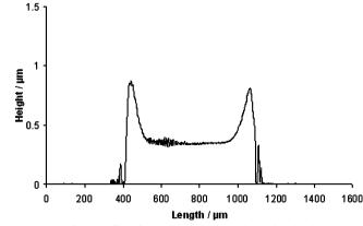
**Fig. 6** Surface profile of an unsintered PZT line printed using 0.6 M PZT sol and electrohydrodynamic atomisation
