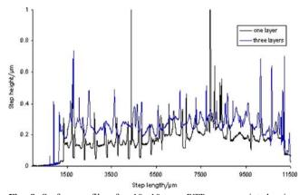
Fig. 8 Surface profile of a  $10 \times 10$  mm PZT square printed using 0.1 M PZT made from one and three layers of 20 lines. The average height of one layer is 185 nm, whilst the average height of the three layered feature is 272 nm
