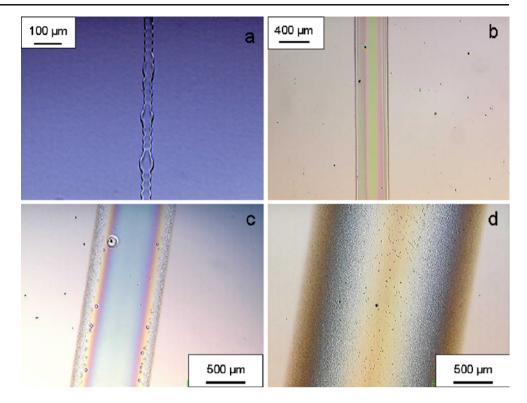
Lines were printed using the EHDA technique from droplets deposited so that they overlap (Fig. 5a). The printing parameters (flow rate and distance between nozzle and wafer) can then be altered to vary the line width (Fig. 5b, c and d). As the line width is increased, the printed structure becomes less continuous and the definition at the edge of the line is decreased (Fig. 5c and d). The surface profile of a cross section of the printed line was investigated (Fig. 6).
