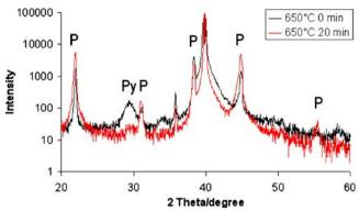
Fig. 3 XRD pattern of propanol-based PZT sol sintered at 650 °C for 0 and 20 min. The pyrochlore (Py) and perovskite (P) phases are indicated
